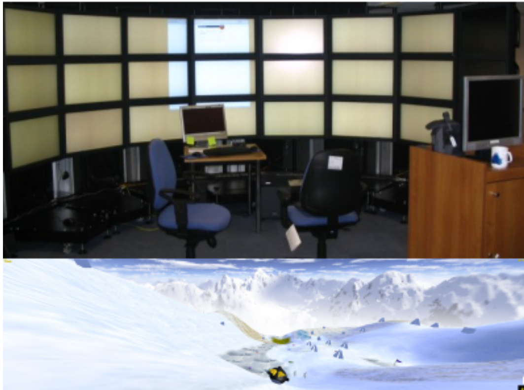
Figure 1: (Above) The visualisation environment in our lab. Each of the monitors are mounted on trussing custom designed to be reconfigurable. (Below) A scaled down view of a 8960 \times 2304 pixel screenshot of the popular Planet Penguin Racer running on the cluster.
